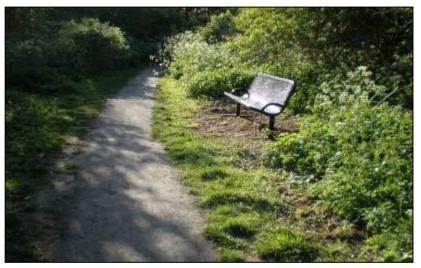
The main circulatory path round the lake is constructed of whinstone dust to fit in with the natural environment of the quarry. Path improvements are ongoing, they are top dressed as required and new construction is installed if desire lines are to be formalised. The paths through the elder woodland are formed with chipped bark and the programme for keeping these in a useable condition is part of the Park Warden role within the Quarry with the additional assistance from volunteers.
